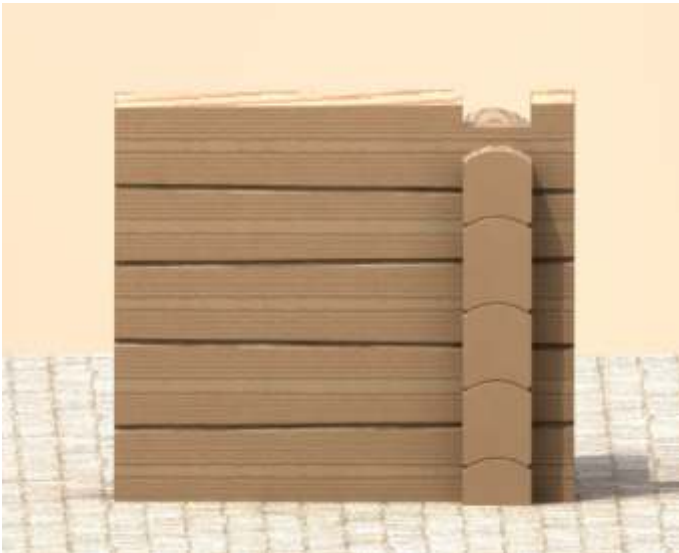
Scandinavian system – view of a side wall with visible compensation of log convergence.
