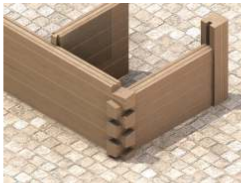
Connection of external wall with internal wall with use of half-interlocking dovetail.
